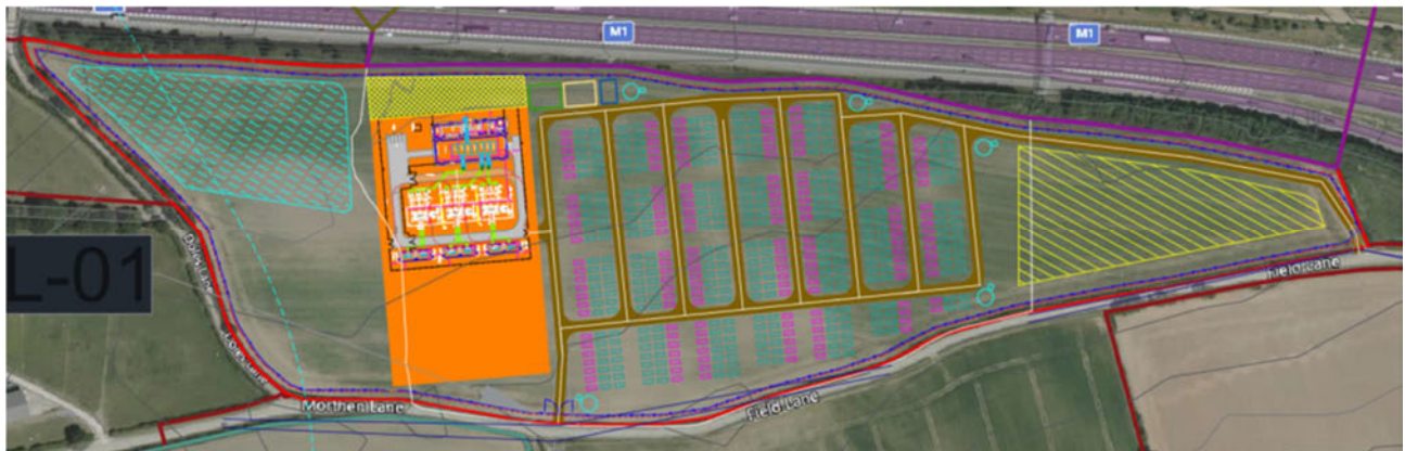
Figure 1.1: Proposed Concept BESS and Substation Layout
